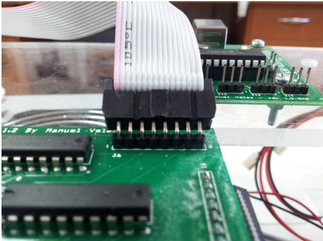
The central connector cable connects to the connector J6 of display 2 using the row of pairs holes in the connector:
